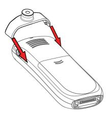
Figure 11. Attach the swivel-type clip into position.
