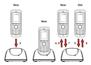
Figure 12. Easy Replacement Procedure via the DC4 Advanced Desktop Charger
