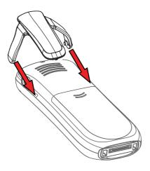
Figure 10. Attach the hinge-type clip into position.
