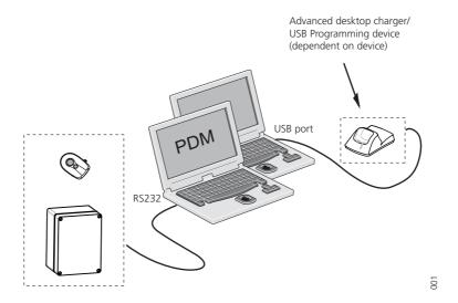
Figure 1. Connection to the PDM depends on device type.
