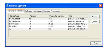
Figure 29. File management window, Parameter definition tab
